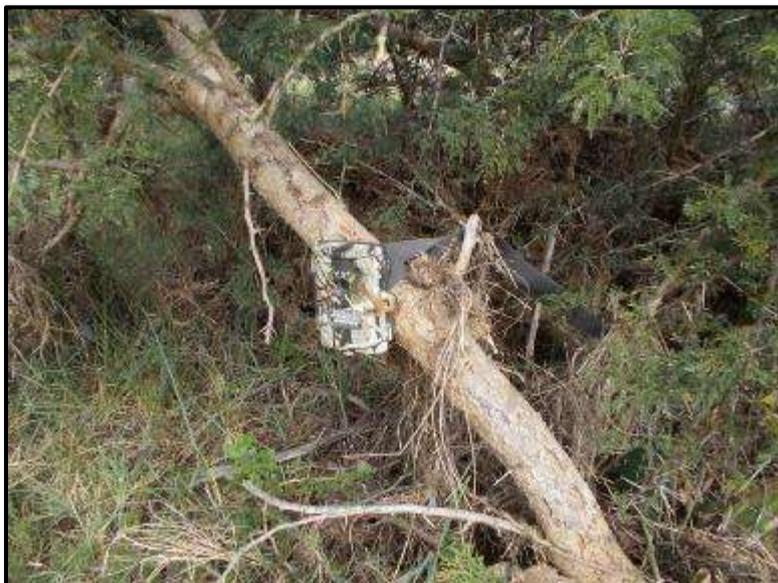
**Figure 8: Infrared camera trap used to observe illusive and nocturnal species.**
